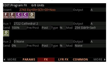
The K2088/61's Chains contain a variety of effects. Each Chain displays icons representing the type of effects contained in the Chain, as well as the order of effects in the Chain (signal flows from left to right). The K2088/61's Chains include different types of reverb, chorus, delay, flanger, phaser, tremolo, panner, rotary, distortion, EQ, compression, filter, envelope following filter, frequency stimulator, ring modulator, frequency offset, pitch LFO, and stereoizer.
