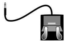
The SW1 (SUSTAIN) and SW2 jacks can be connected to dual switch pedals (2 pedals per jack), allowing up to four switch pedals to be used. Compatible pedals should use a single 1/4 inch tip-ring-sleeve (TRS) plug. (Two single switch pedals can also be plugged into one jack by using a 1/4 inch stereo (male) to dual mono (female) cable, aka TRS male to dual TS female.)
