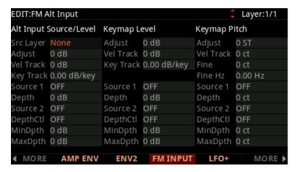
In classic FM synthesis, Operators containing sine wave oscillators are used to frequency modulate other Operators in various configurations in order to create complex timbres. FM layers allow you to use an alternate input for these Operators, allowing sources other than FM Operators to be used for modulation of other FM Operators. This is useful for easily creating complex timbres without complex configurations of Operators and modulation sources.
