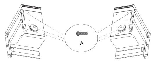
Finish attaching the piano to the stand by using the six Piano Body Bolts (A) to attach the bottom of the piano to its stand.
