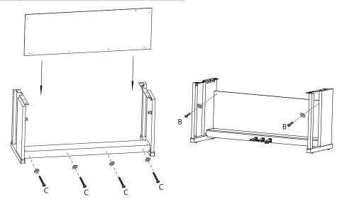
Using four Back Panel Bolts (C) with washers, and two Back Panel Bolts (B) with washers, attach the Back Panel to the stand.
