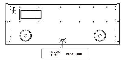
Attach the DC Adaptor and Pedal Cable into their connectors on the bottom of the piano as shown.
