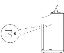
With help from another person, lift the piano onto the stand and slide forwards, pushing the guide rods on the bottom of the piano into the slots on the Stand Legs, as shown below. When lifting the piano onto its stand, be careful not to catch/trap hands or fingers.
