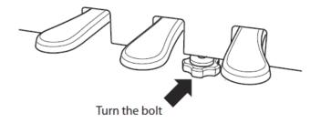
Turn the Pedal Support Bolt beneath pedals counter-clock until bolt firmly rests on the floor.
