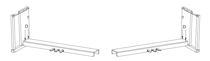
Starting with the right Stand Leg, align the holes in the Pedal Board with the holes in the Pedal Board Bracket as shown. Make sure that the pedals are facing towards the front of the Stand Legs. Thread two Pedal Board Bolts (D) through the Pedal Board and into the bracket. Repeat with the left Stand Leg and tighten all bolts fully.
