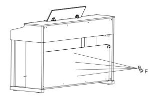
Attach four cable clips(F) to secure the cable.
