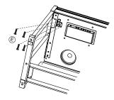
Headphone Holder Installation: Attach the headphone holder to the bottom left of the piano with the four Headphone Holder Bolts (E).
