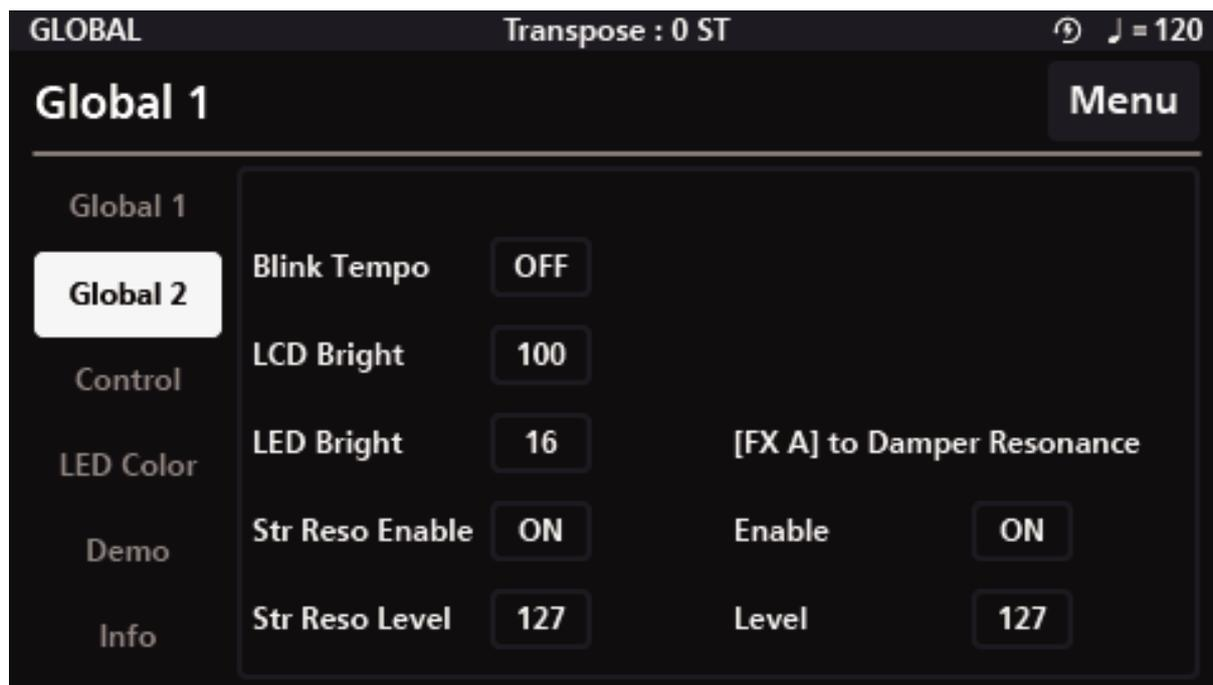
**Blink Tempo:** Enables the Alpha wheel LED ring to “blink” at the current Global BPM tempo value.
