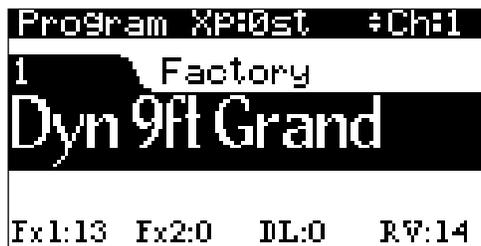
In Program Mode, the top line of the LCD shows the current Mode, MIDI transposition, and MIDI Channel.
