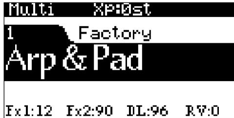
In Multi Mode, the top line of the LCD shows the current Mode and MIDI transposition.
