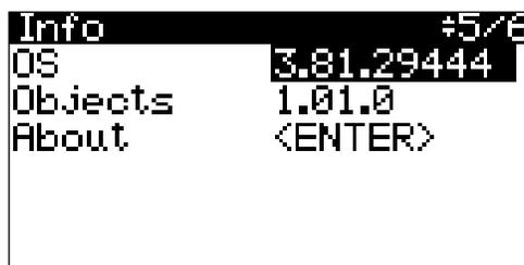
The Info Page shows currently installed Operating System version (OS) and Objects version. To make sure that you have the latest Operating System and sound Objects, go to the Kurzweil website at [www.kurzweil.com](http://www.kurzweil.com).
