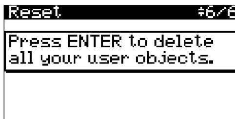
Use the Reset Page to reset the SP6 to its original factory settings. Press the ENTER button to restore all Global Mode settings to their factory defaults, and delete all User Programs and Multis.
