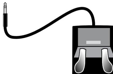
The SW1 (SUSTAIN) and SW2 jacks can be connected to dual switch pedals (2 pedals per jack), allowing up to four switch pedals to be used. Compatible pedals should use a single 1/4 inch tip-ring-sleeve plug.
