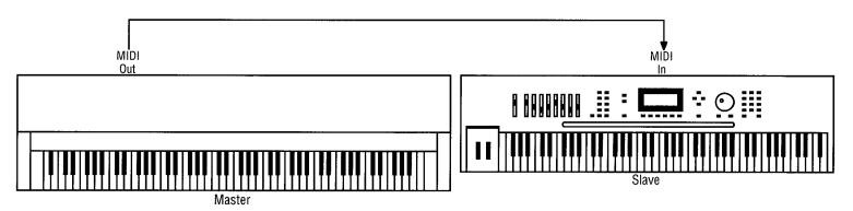
If you connect In to Out, rather than Out to In, the other instrument becomes the master. And if you use two cables, connecting In to Out and Out to In, you can use either instrument as the master.
