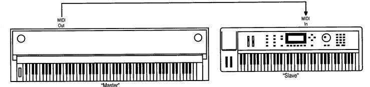
If you connect In to Out, rather than Out to In, the other instrument becomes the master. And if you use two cables, connecting In to Out and Out to In, you can use either instrument as the master.
