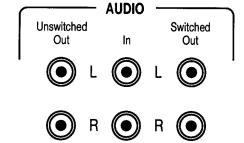
Four RCA jacks provide audio output to external equipment, such as a home stereo, a PA system, or a tape recorder. They are configured in two pairs, each pair consisting of a Left and a Right output for a complete stereo signal. All four provide line-level signals.
