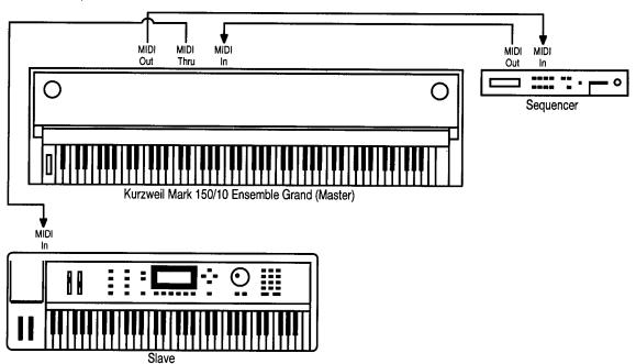
When the sequencer plays back, the information is sent not only to the master, but also—via the Thru port—to the slave. If the slave, in turn, has a Thru port, another slave could be added to the end of this chain, and so on. Practically speaking, though, three or four instruments in a chain are as many as will work effectively; beyond that, transmission becomes unreliable.
