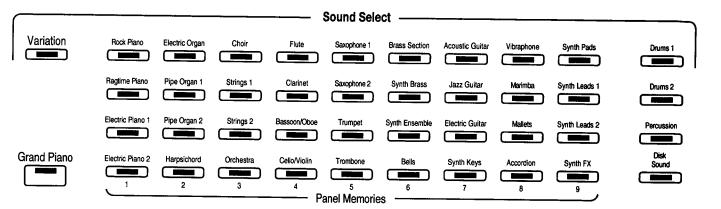
The Sound Select portion of the front panel contains buttons used for selecting the individual sounds available on the Mark 150/10 Ensemble Grand. You select a sound by pressing the corresponding button; the light in the button illuminates to show you which sound is selected.
