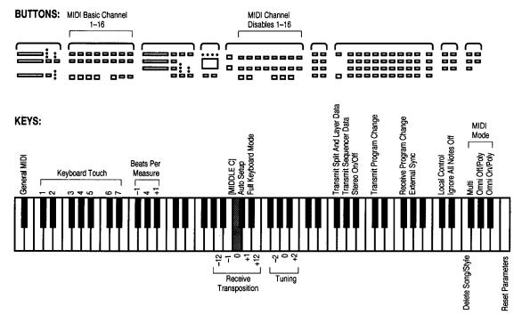
Settings controlled by keys on the keyboard are shown in the Tempo display when the keys are pressed.
