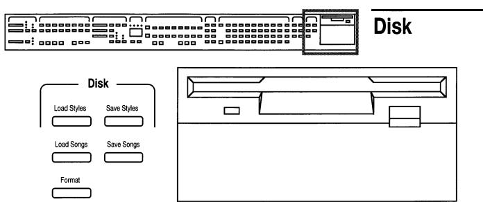
The Mark 150/10 has a built-in high-density disk drive, located at the right end of the front panel. The disk drive allows you to save information onto disks for storage for an indefinite period of time, and to load information from disks into the Mark 150/10. What kind of information? Songs for the Recorder, additional accompaniment styles, SoundBytes<sup>TM</sup>, and Panel Memories.
