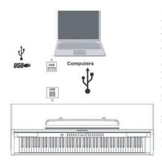
In addition to the conventional MIDI In and MIDI Out ports, the KA150 digital piano also has a USB (Universal Serial Bus) port on the rear panel. You can connect the KA150 digital piano directly to a computer with a USB cable. This connection transmits and receives MIDI data between the KA150 digital piano and the computer.
