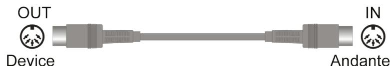
When you connect the MIDI Out of the CUP310 to the MIDI In of another instrument, you can play the sounds of both instruments simultaneously from the CUP310's keyboard. When you connect the MIDI In of the CUP310 to the MIDI Out of another controller, you can control the CUP310 using the other controller.
