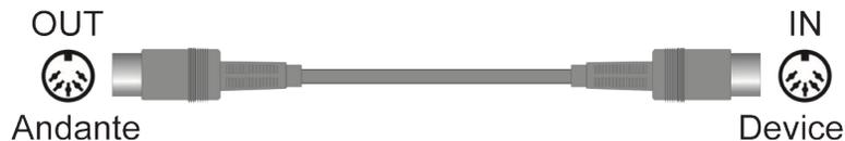
When you connect the MIDI In of the CUP2A to the MIDI Out of another controller, you can control the CUP2A using the other controller.
