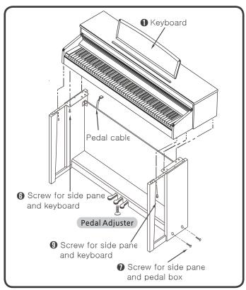
1 Place the Okeyboard on the stand and align with the holes in the side panel brackets.
