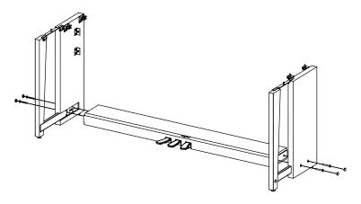
**STEP 2:**Raise the legs and pedals to a standing position, and attach the back panel to brackets, from the rear, as shown below.
