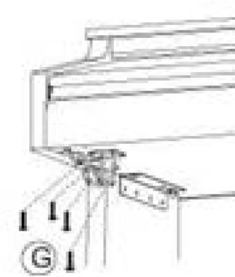
Headphone Holder Installation: Attach the headphone holder to the bottom left of the piano with the four Headphone Bolts(G).
