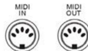
Your instrument MIDI IN connector receives MIDI data from an external MIDI device which can be used to control yours. The MIDI OUT connector transmits MIDI data generated by your instrument (e.g. Note and velocity data produced by playing the keyboard).
