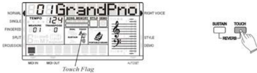
Press [TOUCH] button, you can turn ON/OFF the touch function. When the touch function is ON, the volume will be varied according to how hard you play on the keyboard.
