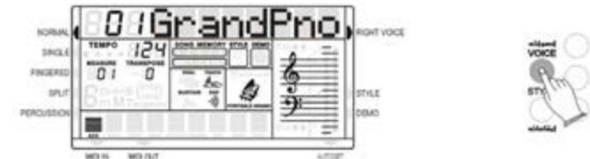
Press the numeric key-pad buttons, or the [+/-] buttons to select the desired voice number according to the Voice List.
